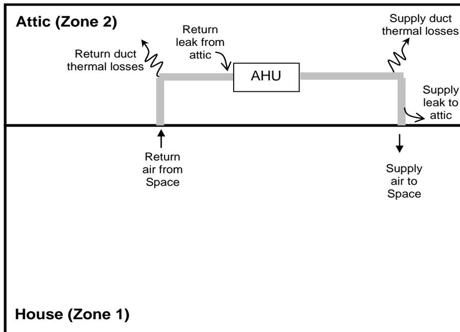
Figure A1. Schematic representation of duct leakage in a home with attic ducts
