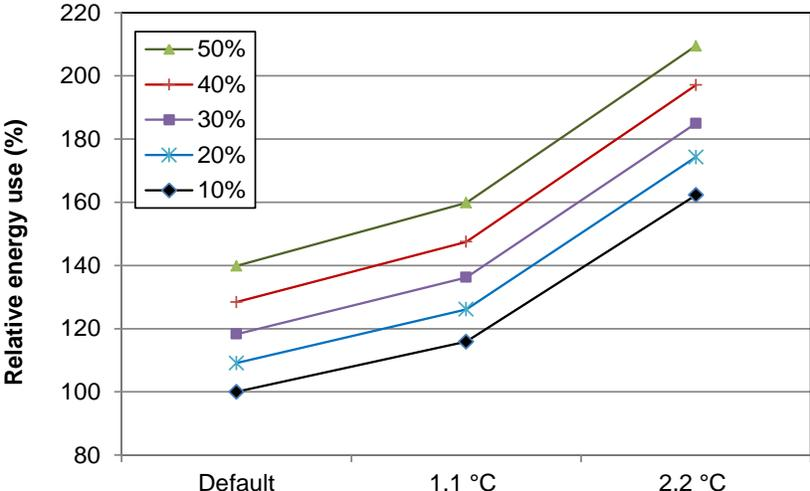
Figure 5.4. Energy use for a slab-on-grade house in Houston with duct leak rates from 10 % to 50 % at three thermostat set point temperatures related to energy use for the house at the default set point and 10 % leak rate (shown in Table 5.9)
