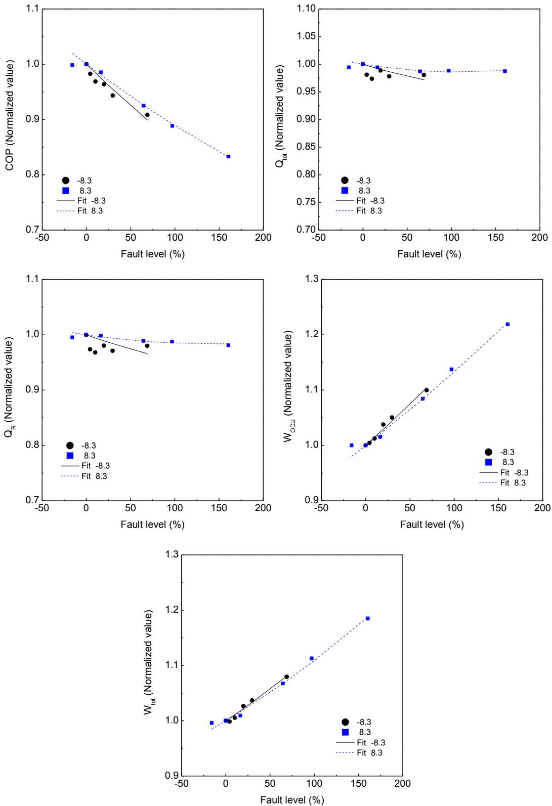
Figure 3.12. Normalized heating performance parameters for improper refrigerant subcooling
