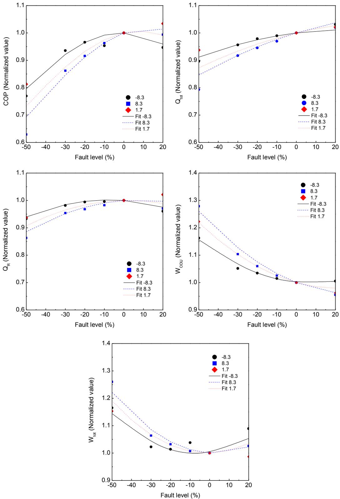
Figure 3.9. Normalized heating performance parameters for improper indoor airflow
