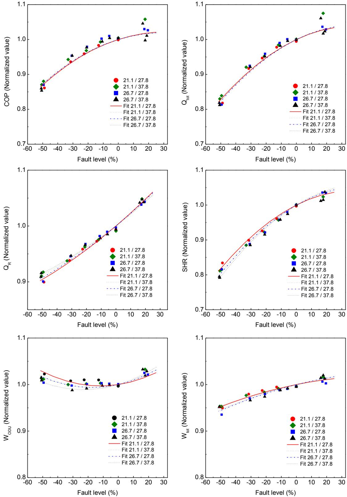
Figure 3.3. Normalized cooling performance parameters for improper indoor airflow
