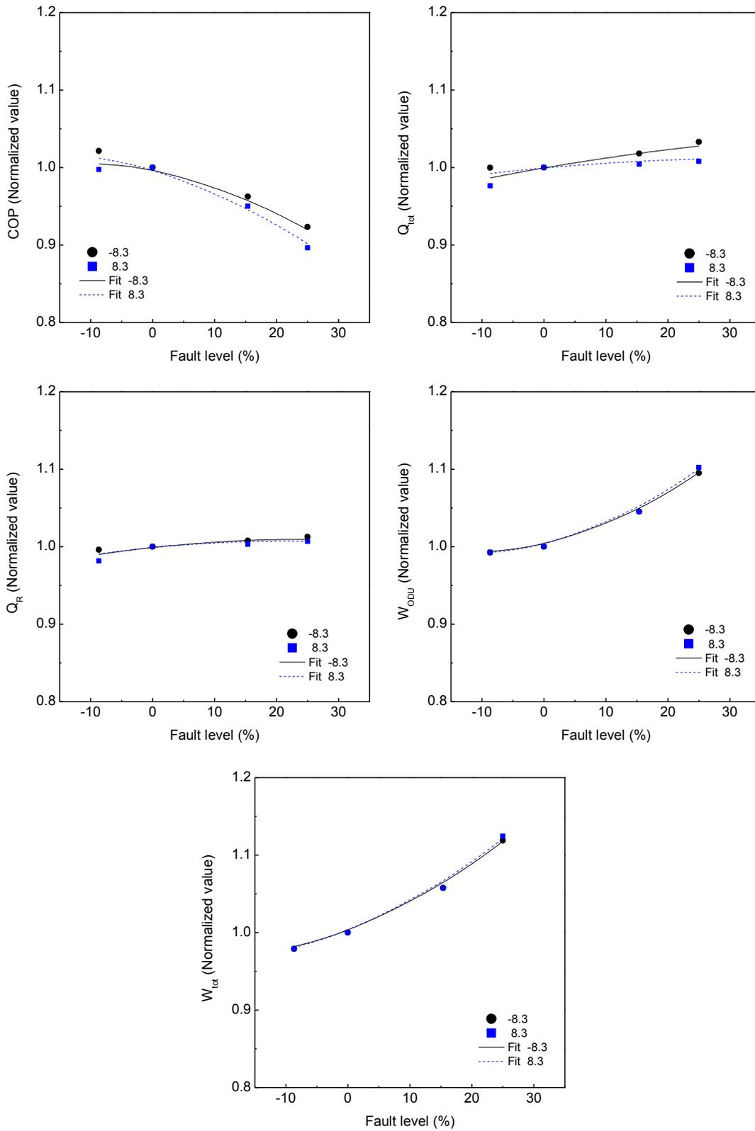
Figure 3.14. Normalized heating performance parameters for improper line voltage
