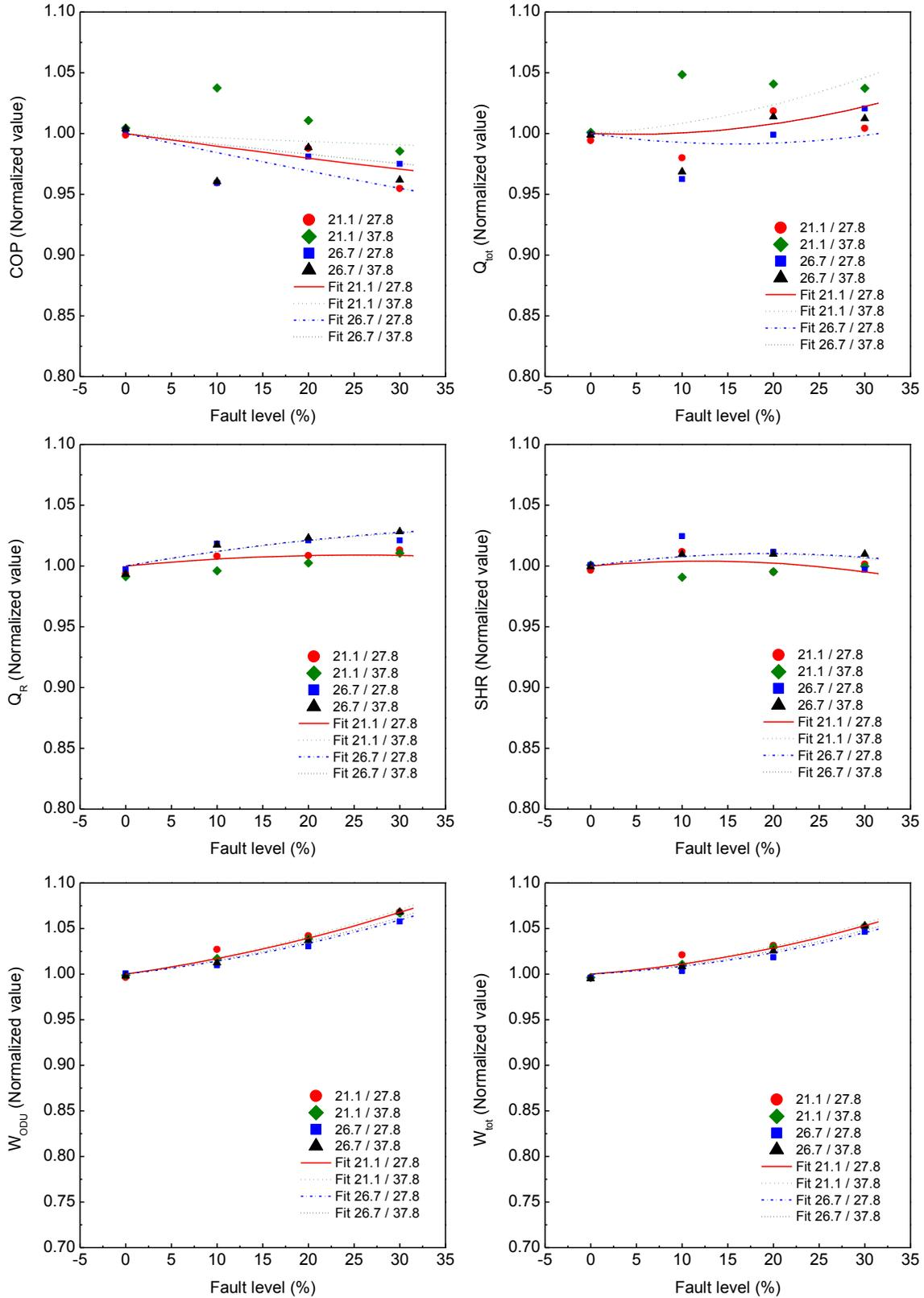
Figure 3.5. Normalized cooling performance parameters for refrigerant overcharge
