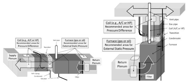
Note: For purposes of these Figures, the filter is included as part of the OEM box and therefore part of the pressure drop across the equipment.
