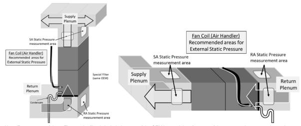
Note: For purposes of these Figures, the filter is included as part of the OEM box and therefore part of the pressure drop across the equipment.
