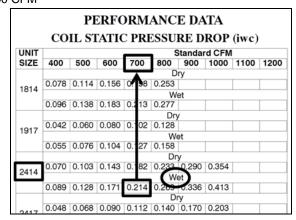
Note: For altitudes greater than 2,500 feet above sea level, calculated ESP needs to be corrected for elevation (i.e., air density impacts) before using OEM-provided performance data. Most OEM data is based on standard air
